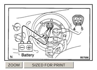
e. If you have no TOYOTA hand-held tester, connect the positive (+) lead from the battery to terminal 4 of the connector, and the negative (-) lead to terminal 5.
