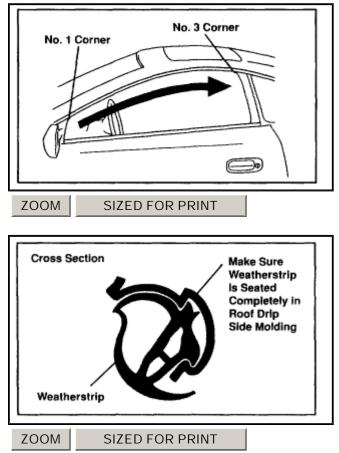
5. Using finger pressure, press the length of the weatherstrip between the No. 1 and No. 3 corners to verify that the weatherstrip is seated completely in the roof drip side molding as shown in illustration.
