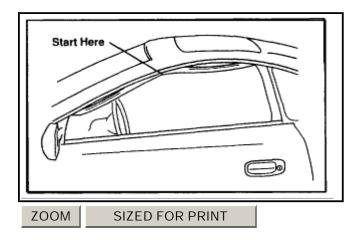
2. If the weatherstrip is in good condition, start by installing the weatherstrip in the No. 2 corner. If the weatherstrip is damaged, replace the weatherstrip.
