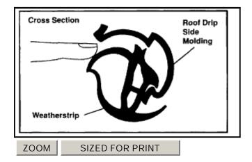
3. Hook the bottom edge of the weatherstrip into the roof drip side molding first. Then, using your fingers, install the top edge of the weatherstrip into the molding.
