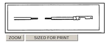
B. Securely attach a 45 cm/18 in wire with an outside diameter of 2.0 mm or larger to the tail of the new terminal.
