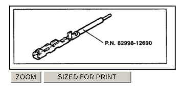
A. Order a new terminal with lead that is the same size and type as the terminal previously removed from the connector. (PN 82998-12690)
