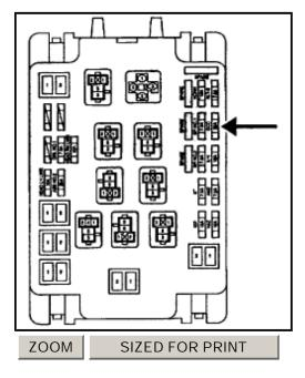
If a vehicle exhibits this condition, check that the DCC 25 amp fuse is in the Junction Block as shown.
