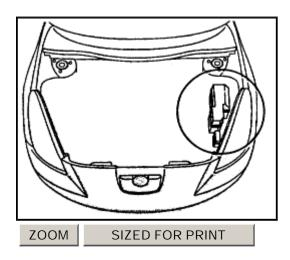
The DCC 25 Amp fuse is stored in the Engine Room Junction Block in the engine compartment. Refer to TSB PG027-99 for Celica Fuse Installation During POS.
