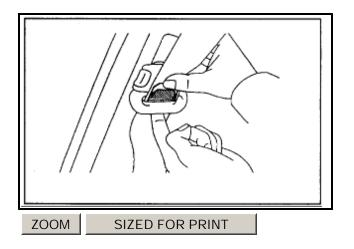
B. By pulling up the <u>seat belt</u>, put the fluorocarbon resin tape through the hole of the shoulder belt anchor. Match the shoulder belt anchor to the center of the tape.
