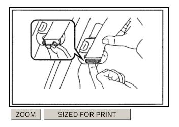
D. Remove the lower side colored film from the fluorocarbon resin tape, and securely affix the tape to the outside of the shoulder belt anchor.
