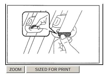
C. Remove the upper side colored film from the fluorocarbon resin tape, and securely affix the tape to the outside of the shoulder belt anchor.
