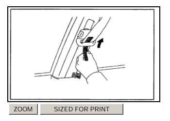
B. Put the Velcro tape (in the parts kit) through the hole of the shoulder belt anchor, brush-shaped side to the anchor.
