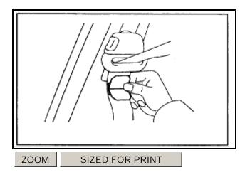
A. Place the fluorocarbon resin tape onto the <u>seat belt</u> as shown in the illustration.
