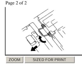
A. Release the spring between the No.1 and No.2 sunshades on both sides.
