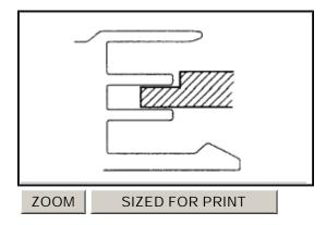
HINT: When re-installing the sunshade, insert it into the slider rail as shown.
