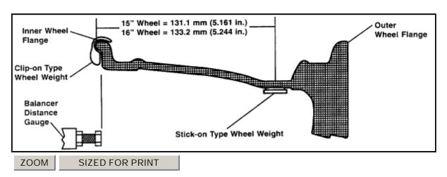
1. Mount tire/wheel assembly on wheel balancer with the outside or decorative wheel flange opposite the wheel balancer arbor.
