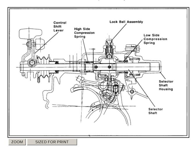
3. Remove the Selector Shaft by removing the Control Shift Lever, Lock Ball Assembly and the 4 bolts for the Selector Shaft Housing (MX-13 & MX-14, Steps 7, 8, & 10).
