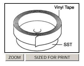
b. Wind a vinyl tape around SST at the place **4.0 mm (0.157 inch)** above from the bottom end until the thickness of the wound tape is about **5.0 mm (0.197 inch).** SST 09950-60010 (09951 -00320) **NOTICE:** Clean SST to remove deposited oil, before winding a vinyl tape.
