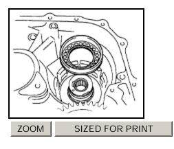
e. Install the U/D brake piston to the transaxle <u>case</u>.
