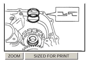
a. Install the 2 oil seal rings to the transaxle <u>case</u>.
