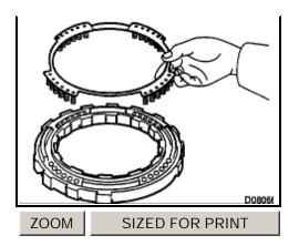
c. Install the return spring to the 2nd brake piston.
