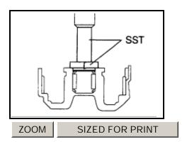
c. Using SST and a press, install the needle -roller bearing to the transaxle <u>case</u>. SST 09950-60010, (09951-00320), 09950-70010 (09951-07100) **NOTICE:** When the wound vinyl tape contacts the transaxle <u>case</u>, stop press-fitting.
