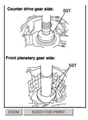
b. Using SST and a press, install the 2 bearing outer races to the transaxle <u>case</u>. SST 09950-60020 (09951-00890), 09950-70010 (09951-07150) **NOTICE:** Press-fit the bearing race until it contacts the snap ring. Do not apply excessive pressure to it.
