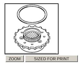
b. Install the thrust washer No.2.
