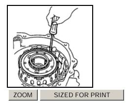
d. Using a screwdriver, install the snap ring.
