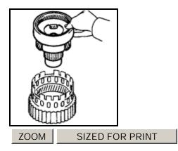
a. Install the front planetary gear to the brake hub.
