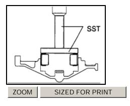
b. Using SST and a press, install the U/D cylindrical roller bearing. SST 09950-60020, (09951-00810), 09950-70010, (09951-07100) **NOTICE:** Do not apply excessive pressure to it.
