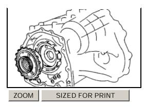
c. Install the rear planetary gear from the rear planetary <u>ring gear</u>.
