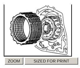
a. Install the 5 plates and 5 discs.
