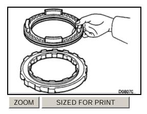
b. Install the 2nd brake piston to the 2nd brake cylinder.
