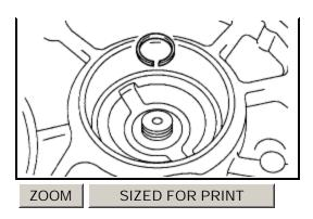
a. Install the oil seal ring to the transaxle housing.
