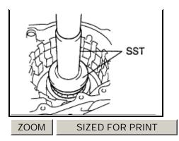
d. Using SST and a press, install the counter drive gear and bearing to the transaxle <u>case</u>. SST 09950-60010 (09951-00890), 09950-70010 (09951-07150) **NOTICE:** Do not apply excessive pressure to it.
