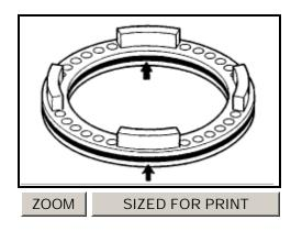
a. Coat 2 new O-rings with <u>ATF</u>, install them to the 2nd brake piston.
