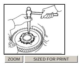
g. Using a chisel and hammer, stake the lock washer.
