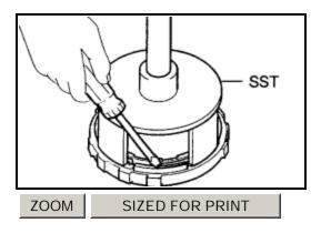
d. Using SST, a press and a screwdriver, install the snap ring. SST 09387-00060
