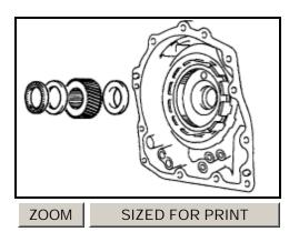
h. Install the 2 bearings, 2 races and front planetary sun gear to the front planetary gear.
