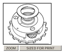
a. Coat a bearing race with <u>ATF</u>, install it to the rear planetary gear assembly.
