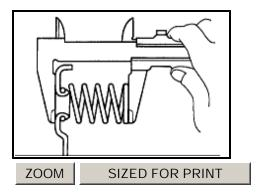
f. Using vernier calipers, measure the free length of the spring together with the spring seat. Standard free length: 13.24 mm (0.5212 inch)
