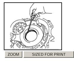
a. Using a screwdriver, install the snap ring to the transaxle <u>case</u>.
