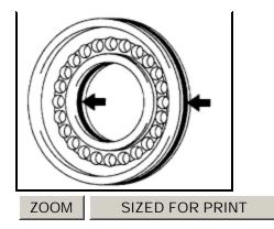
d. Coat 2 new O-rings with <u>ATF</u>, install them to the U/D brake piston.
