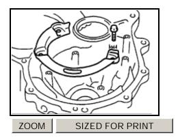
1. INSTALL OIL SEPARATOR Install the oil separator with the 3 bolts to the transaxle housing. Torque: **9.8 Nm (100 kgf-cm, 7 ft. lbs.)**
