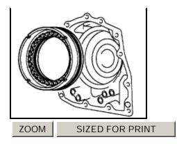
c. Coat a 1st & reverse brake piston with <u>ATF</u>, install the 1st & reverse brake piston to the transaxle <u>case</u>.
