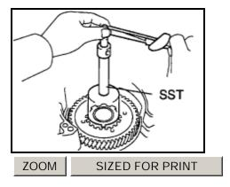
f. Using SST and a torque wrench, measure the starting torque of the bearing. When the measured value is not within the specified value, gradually tighten the nut until it reaches the specified value. SST 09387-00080 Starting torque:
